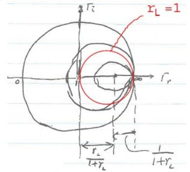
Each of these circles represent all  $\Gamma = \Gamma_r + j\Gamma_c$  that correspond to a given  $r_L$ .
