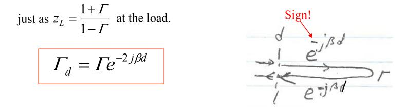
$\Gamma_d$  is just phase-shifted by  $-2\beta d$  from  $\Gamma$ . Therefore,  $|\Gamma_d| = |\Gamma|$ . Just rotate from  $\Gamma$  by  $2\beta d$  clockwise.
