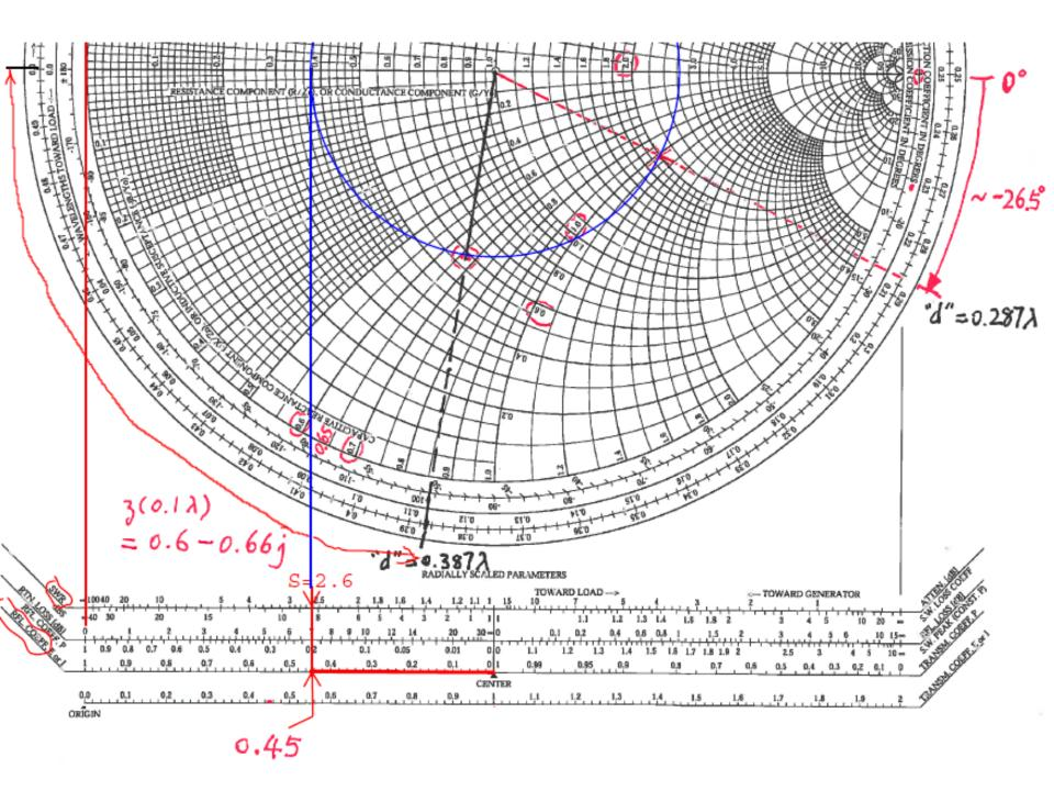
We now move further, and hit the horizontal axis. Recall that on this axis, x(d) = 0,
